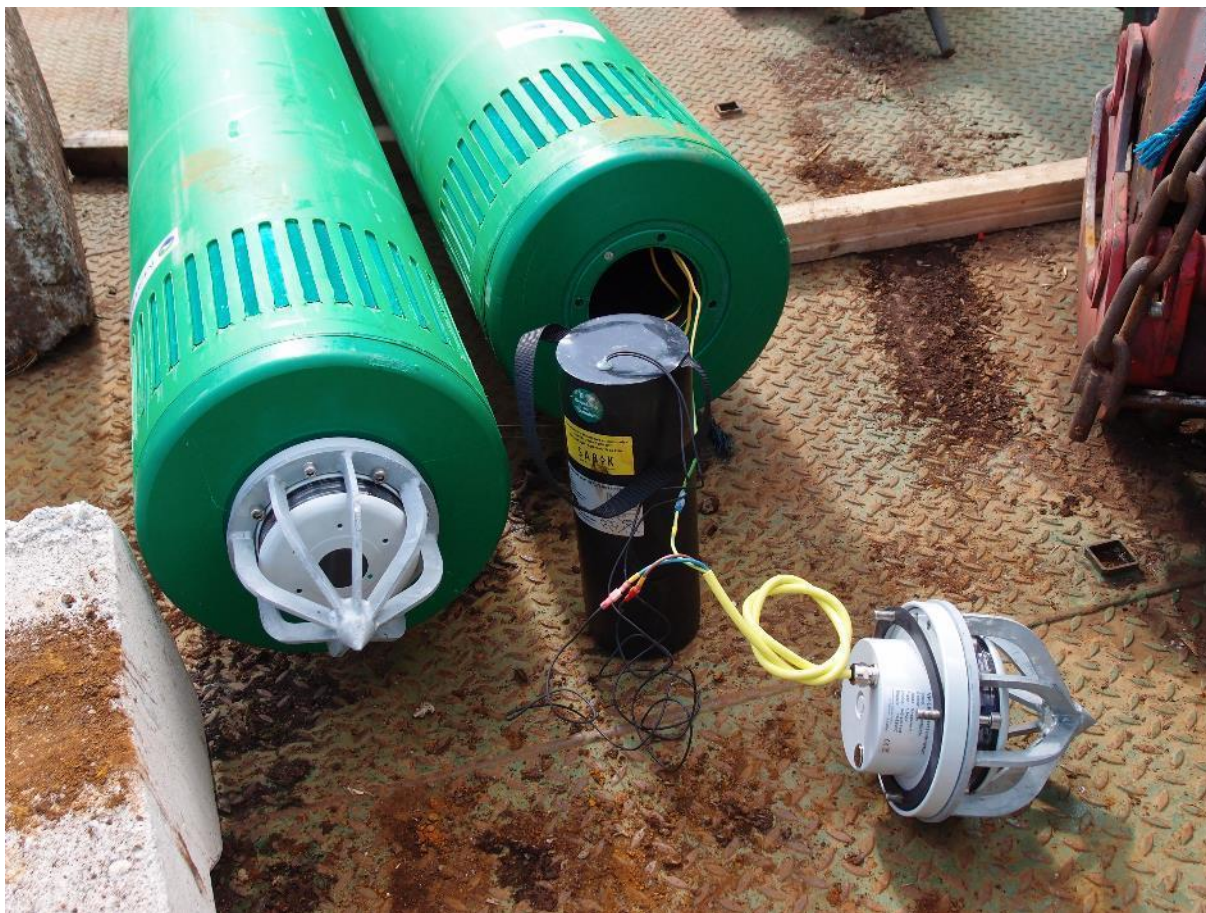
Figure 13 Two smart buoys installed on the pilot fairway, with a battery and light device
