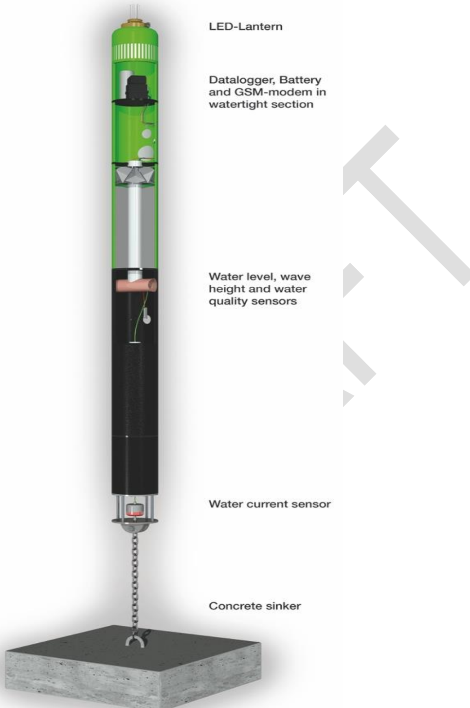
Figure 12: Cross-section of a smart buoy
