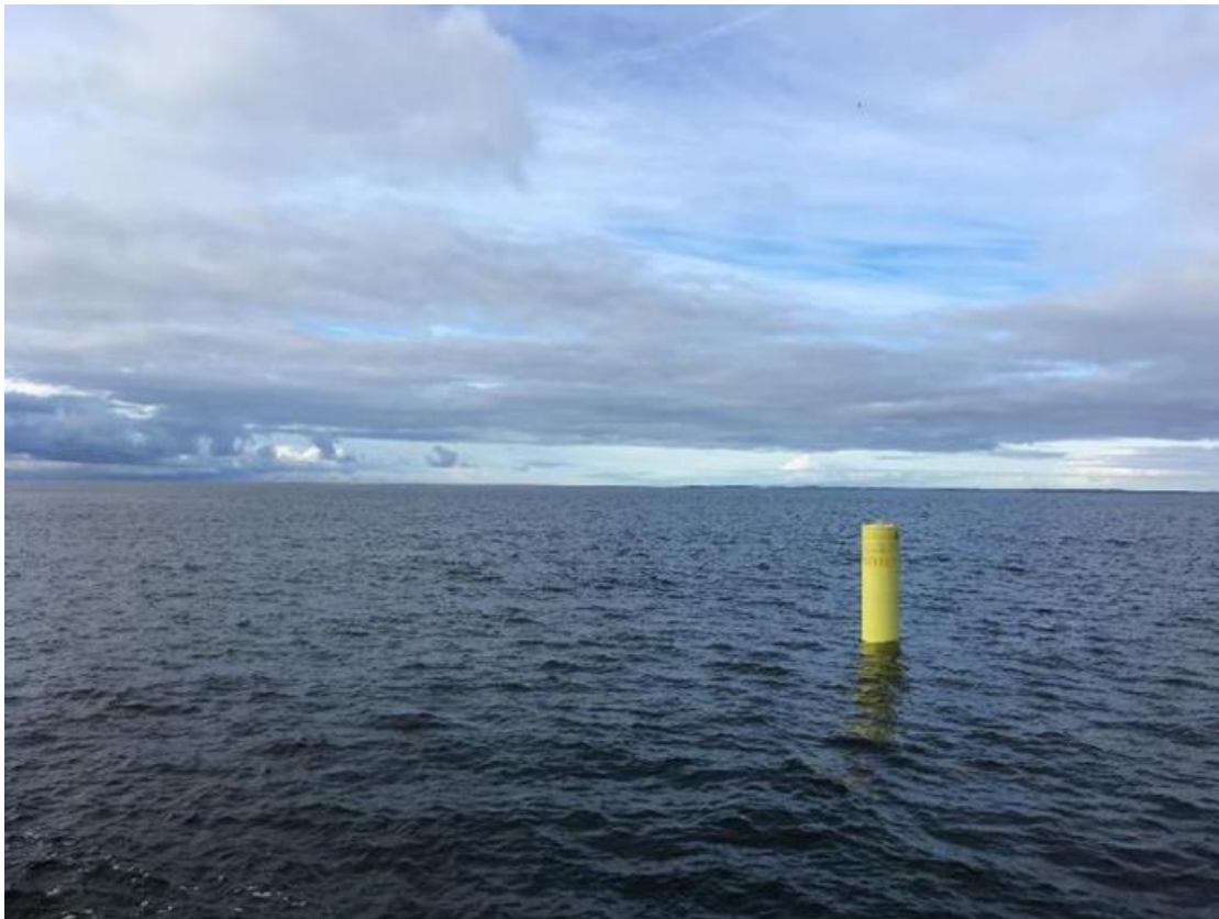
Figure 19 An oil spill detection buoy
