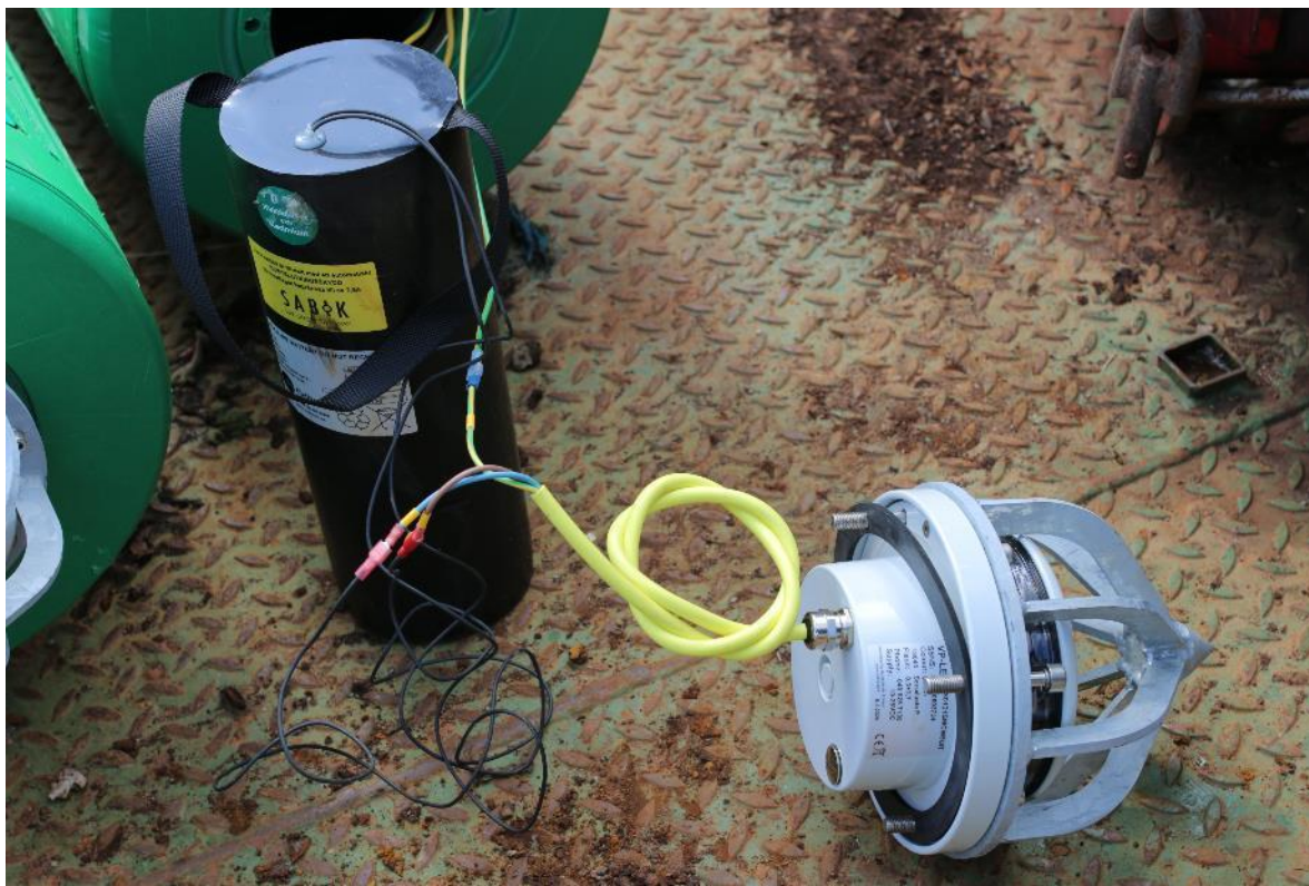
Figure 16: Battery and light device of one smart buoy installed on the pilot fairway
