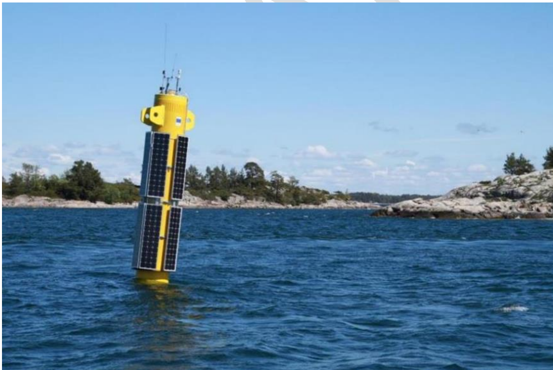
Figure 18 A sniffer buoy measures vessel emissions
