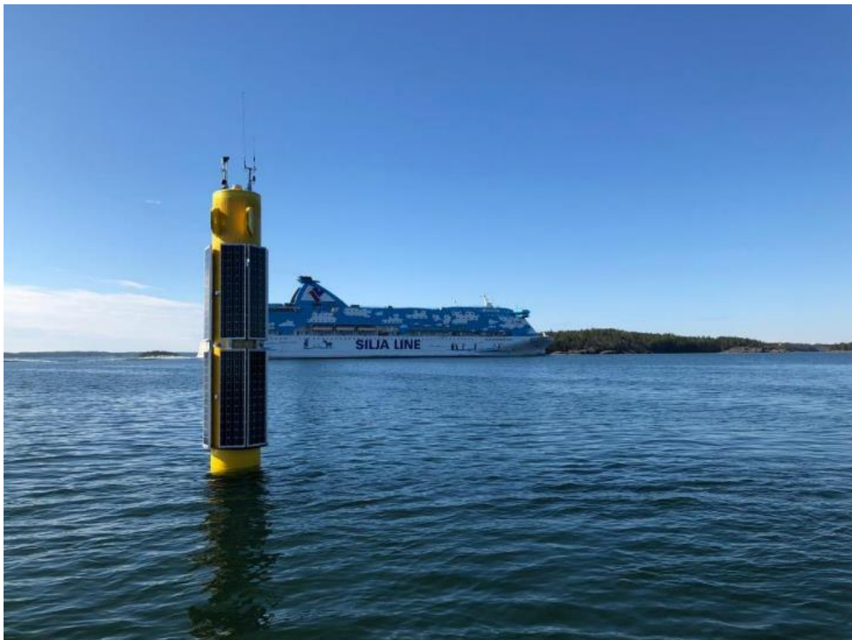
Figure 2: A sniffer buoy with a Finnish cruise ship in the background
