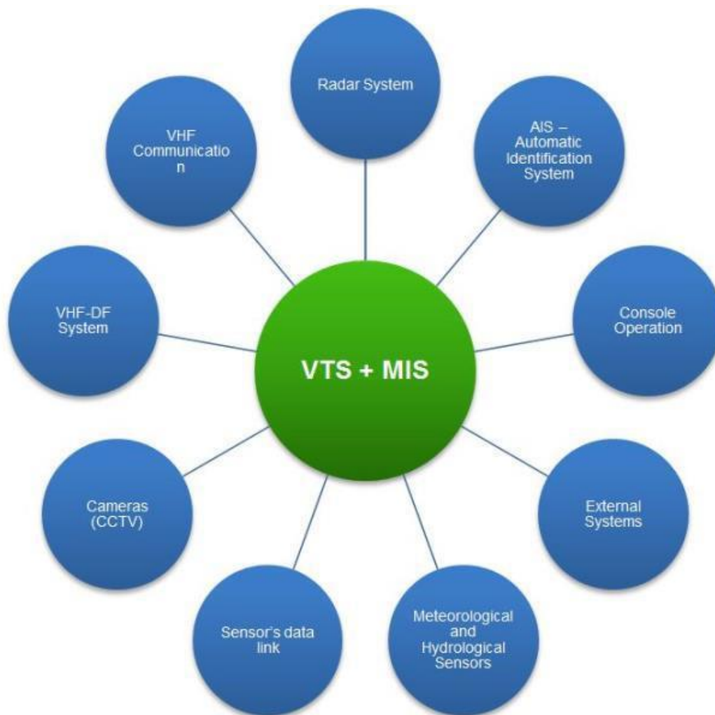
Figure 26: Diagram showing VTMS input and output components and subsystems
