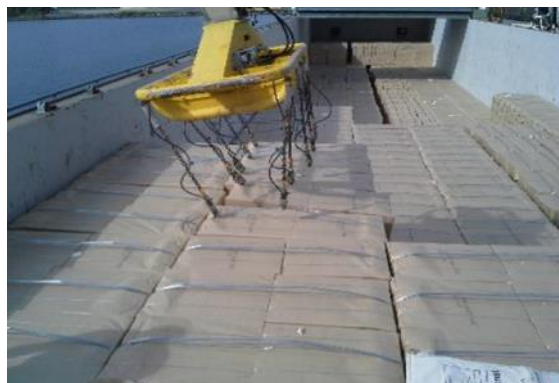
Figure 9: Semi-automatic loading equipment and dissolving pulp bales
