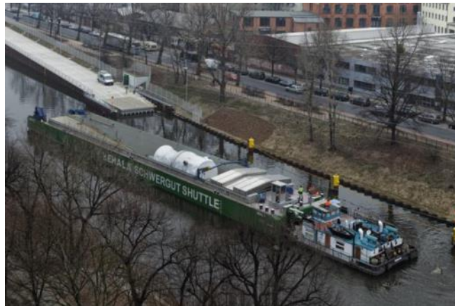
Figure 2: Barge “URSUS” with turbine on the trip from ramp to port
